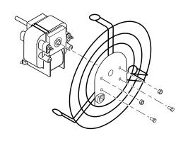
Figure 12 - Removing or Attaching Fan Guard from Motor
